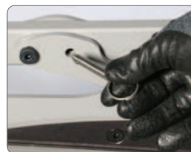
After securing the blade lock-pin in place, the SCSRC1 stone coated roofing cutter is safe to carry on to the job site.
