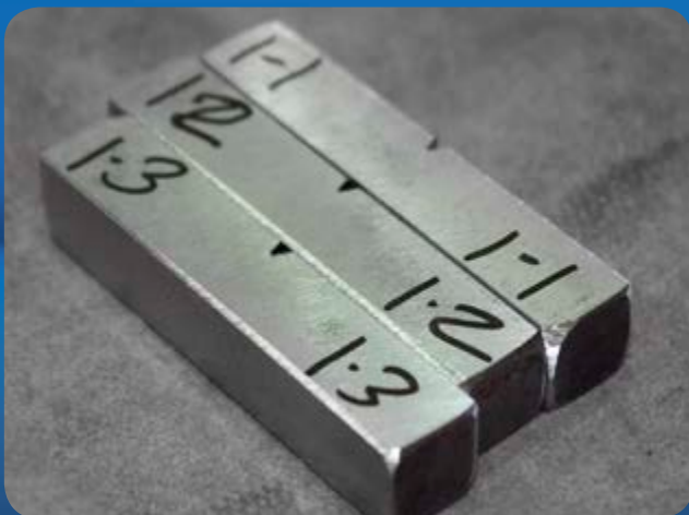
Machined Charpy V-notch samples are ready for testing
