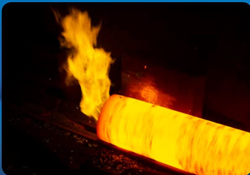
Hot shell moving through a second piercing to increase diameter and length
