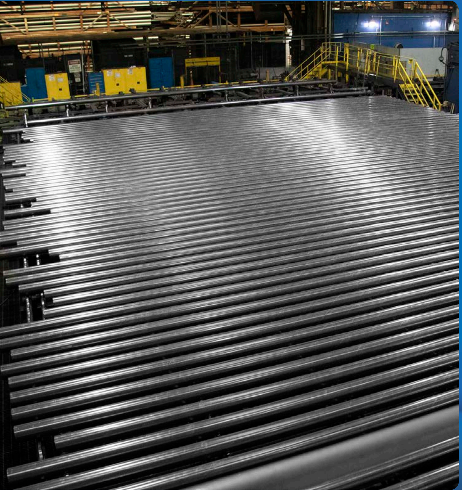
Small OD line pipe on cooling bed after going through the tempering furnace
