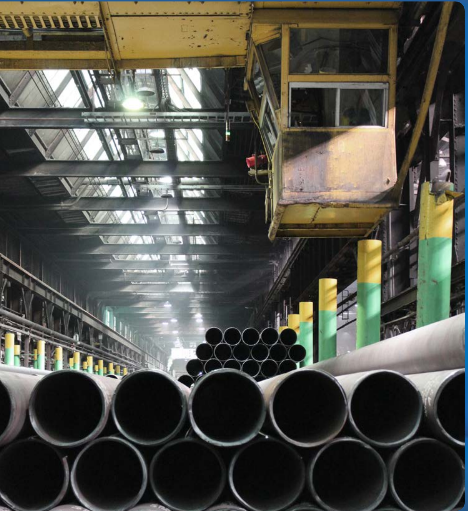
Pipe stored inside Lorain Tubular Operations No. 3 mill waiting for finishing and inspection
