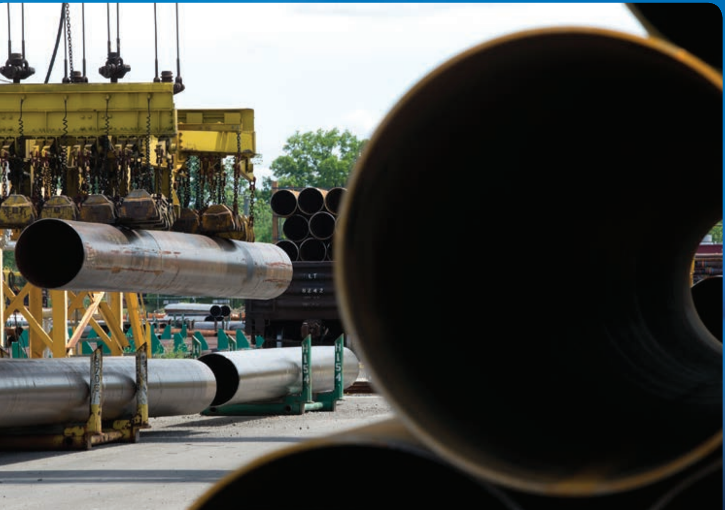
Large line pipe transported by magnetic crane at our Lorain Tubular Operations
