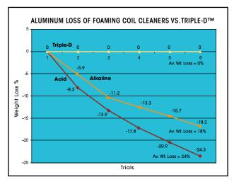
Conventional foaming acid and non-acid coil cleaners attack and chemically react with the aluminum coil components. This reaction is exhibited by a foaming action. The attack/reaction dissolves the aluminum, destroying the heat-transfer ability of the coil and creating the potential for refrigerant leaks.
