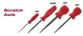
Use to scribe lines on metal, plastic, and a variety of other materials. Pierce holes in wood, plastic, leather - even light gauge metal. Blades are high carbon, alloy tool steel fully polished to resist rust. Blade tapers to a fine point and may be resharpened many times. Easy-to-spot orange handles are shock and shatter resistant.
