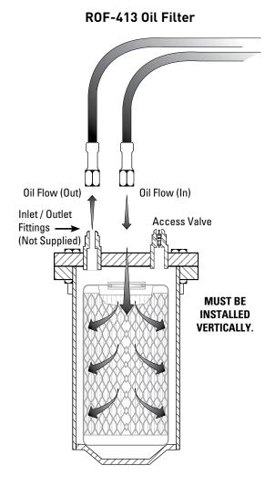
**3**. For the **ROF-413-T**, after the appropriate shut-off valves are tightly closed, relieve system pressure by using the access valve on ROF-413-T end plate. Remove the end plate.
