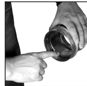
Figure 5: Check for EPDM seal
