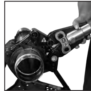
Figure 8: Placement of adapter jaw into pressing chain
