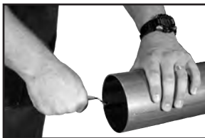
Figure 3: Deburr inside diameter deburring tool
