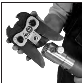
Figure 7: Placement of adapter jaw into the tool
