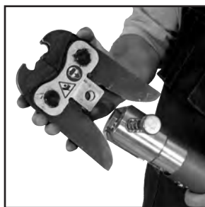
Figure 7: Placement of adapter jaw into the tool
