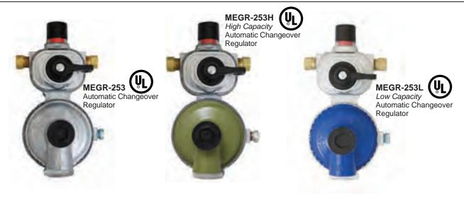
The MEGR-253 Series Automatic Changeover regulators automatically redirect LP gas vapor flow from an empty service cylinder to a reserve cylinder, without interruption of service. It features an easy to read green indicator which changes to red when the service cylinder needs to be refilled.
