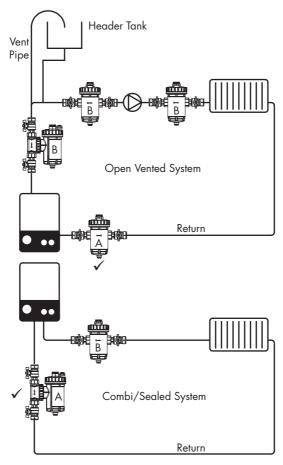
In both diagrams, position A is best practice whilst position B is also suitable
