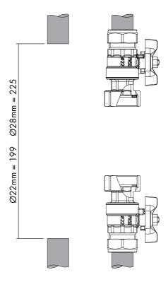
Having removed the prescribed section of pipework, make sure that the open ends of both pieces are free of debris and ready to receive the nut and olive. Fit both isolation valves but do not tighten fully.
