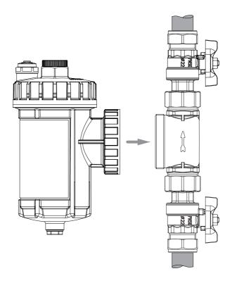
Present the filter to the connector block ensuring the air bleed is at the top and the drain plug is at the bottom. Gently push the filter into the connector block and when you are satisfied with the position of the filter, hand tighten. If further tightening is required, gentle pressure can be applied with a suitably sized set of pump pliers.
