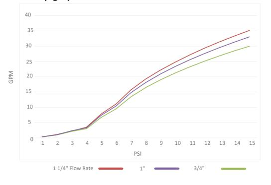
Pressure drop graph Intaklean Flow Rate
