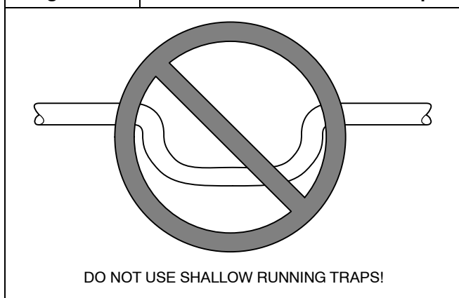
Figure 15 Insufficient Condensate Trap
