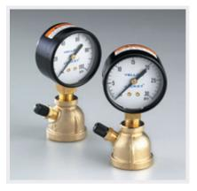
Easy-to-read gauge to test system pressure for leaks in new installations. Pressure drop indicates leakage. 0-30 gauge is in 1/4 lb. increments and 0-15 gauge is in 1/5 lb. increments. Brass threaded bell for leak tight connection.
