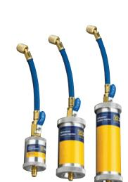
Body and cap are rugged aluminum with an "O" ring seal. 1/4" Male fitting at one end with Schrader. A ball valve for control on other end with a short length of hose. Valve depressor in 1/4" Female end. 600 psi working pressure.
