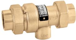
The backflow preventer with atmospheric vent is designed to protect drinking water systems from the return, caused by backsiphonage or backpressure, of contaminated fluids.
