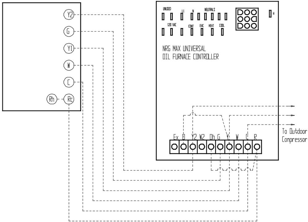
**Heat Pump (1) Stage Heat (1) Stage Cool PSC Motor - Furnace Auxiliary Heat**
