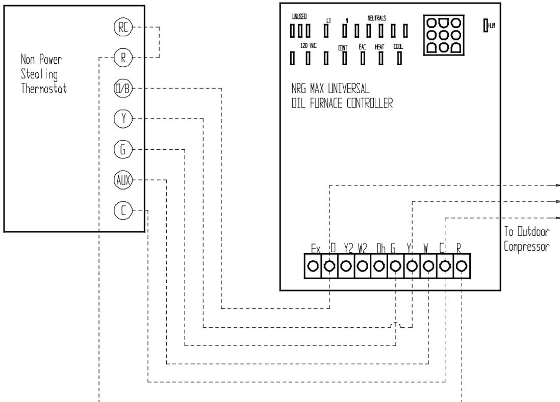
**Heat Pump (1) Stage Heat (1) Stage Cool ECM Motor - Furnace Auxiliary Heat**
