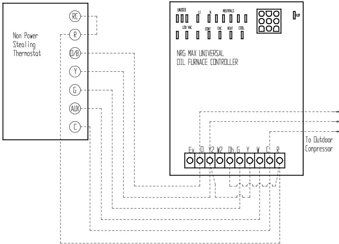
**Heat Pump (2) Stage Heat (2) Stage Cool ECM Motor - Furnace Auxiliary Heat**
