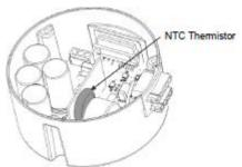
5. Inspect capacitors inside of control unit for bulging or swelling. Replace control unit if capacitors are bulging or swollen
