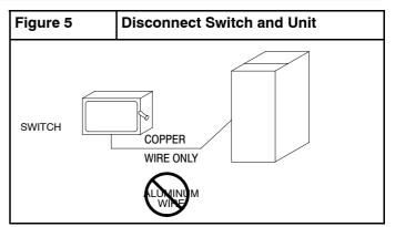
Units Without Factory–Installed Disconnect — When installing units, provide a disconnect switch per NEC (National Electrical Code) of adequate size. Disconnect sizing data is provided on the unit informative plate. Locate on unit cabinet or within sight of the unit per national or local codes. Do not cover unit informative plate if mounting the disconnect on the unit cabinet.
