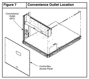
Non-powered type: This type requires the field installation of a general-purpose 125-volt 15-A circuit powered from a source elsewhere in the building. Observe national and local codes when selecting wire size, fuse or breaker requirements and disconnect switch size and location. Route 125-v power supply conductors into the bottom of the utility box containing the duplex receptacle.
