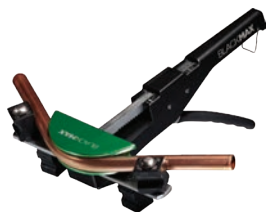
Forward bend configuration
