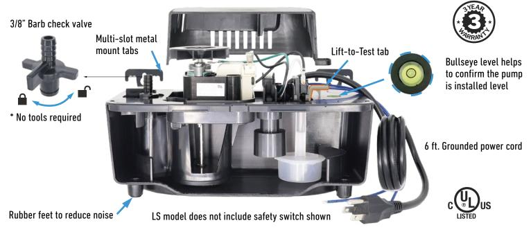
New design offers a longer 3 year warranty life and reduced noise level. Includes lid mounted bullseye level for easy installation. Rated for condensate water up to 150° F. Automatic start/stop operation with thermally protected motor. More water pumped out per cycle means the pump runs less and lasts longer. Larger 2.5 quart tank capacity.
